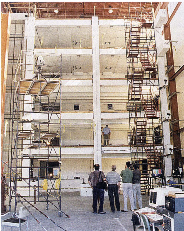
Fig. 5. Test building is 30 ft wide and 40 ft high (9.1 x 12.2 m).
