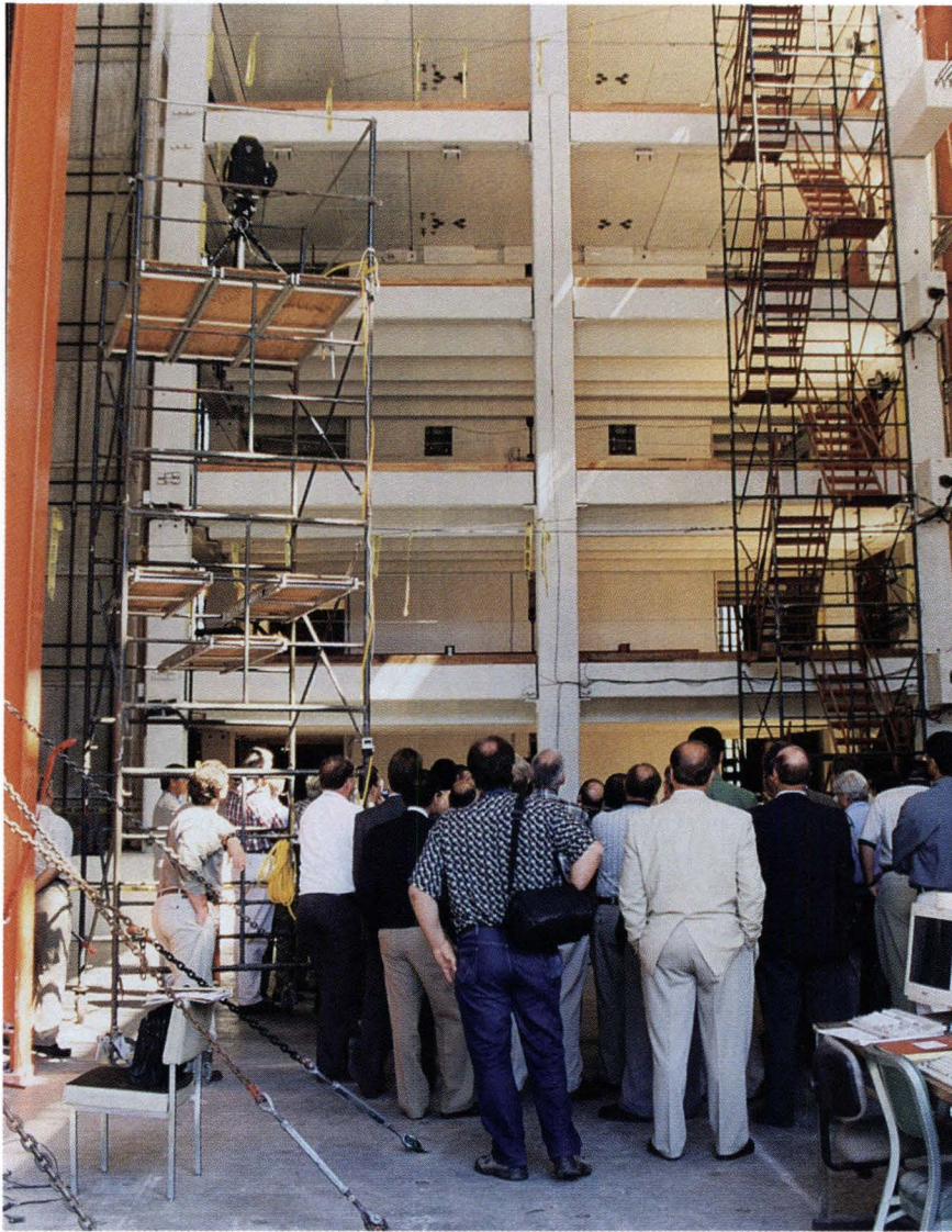
Fig. 1. Over 60 people witnessed the seismic testing of a five-story precast, prestressed concrete building at the University of California, San Diego.
