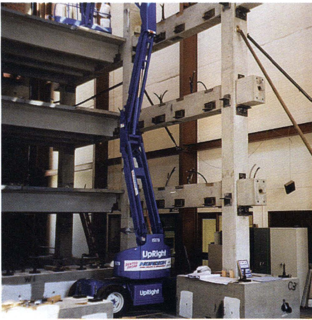
Fig. 3. Hybrid frame under construction.
